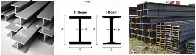
The Parallel Flange Beams come in different shapes depending upon the width & depth of the beam and are generally known as I-beam and H-beam. The H-beam has wider flanges than an I-beam, while the I-beam has tapered edges. Thus the main difference between both H-beams and I-beams is the flange by web ratio. The types beams further vary
