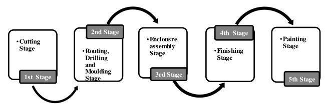
• **Cutting Stage** – This is the initial stage of loudspeaker manufacturing process. At this stage plywood or MDF Sheet is cut into required shapes and sizes according to different models.
