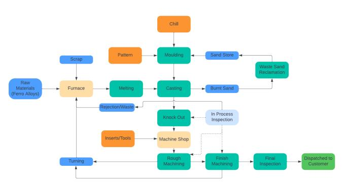
The raw materials and steel scrap are melted in the furnace and the accurate chemical composition is achieved. This liquid metal is then poured into a sand mould. Once cooled, the 'knockout' process begins, involving the removal of sand and moulds to reveal the raw casting. The castings then undergo initial inspection for any flaws or defects, with faulty castings being either repaired or recycled.
