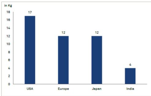
The penetration of sintered component per vehicle in India is estimated at 4 kilogram per vehicle, which is significantly lower than that in global counterparts as detailed in the chart below.
