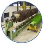
Flight welding machine for 4500 mm diameter x 24,000 mm length
