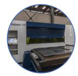
Laser Cutting Machine for plates upto 16 mm thick
