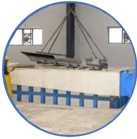
Bath pickle stainless steel jobs up to 6000 x 2000 x 2000mm size
