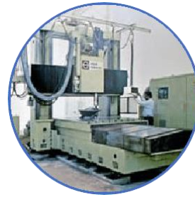
Machine job with maximum size of upto 10,000 x 4000 x 1000 mm on CNC Machines
