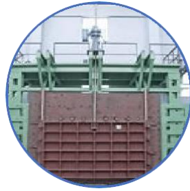
Hydro-test sluice gates up to 5000 x 3500mm size and valves up to 3000mm
