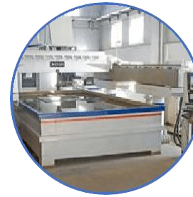
Water jet Cutting of stainless steel plates upto 100 mm thick
