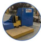
Flight Forming Machine for 5000 mm diameter
