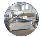
Water jet Cutting of stainless steel plates upto 100 mm thick
