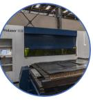
Laser Cutting Machine for plates upto 16 mm thick
