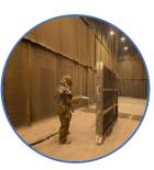
Shot blasting of carbon steel up to 5000 x 4000 x 20000mm
