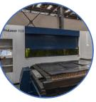
Laser Cutting Machine for plates upto 16 mm thick
