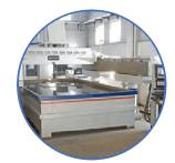
Water jet Cutting of stainless steel plates upto 100 mm thick
