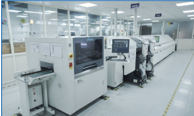
Automated SMT mounting & solder-paste printing
