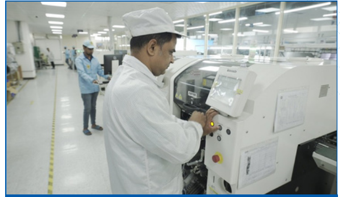
Precision component placement under clean-room protocol
