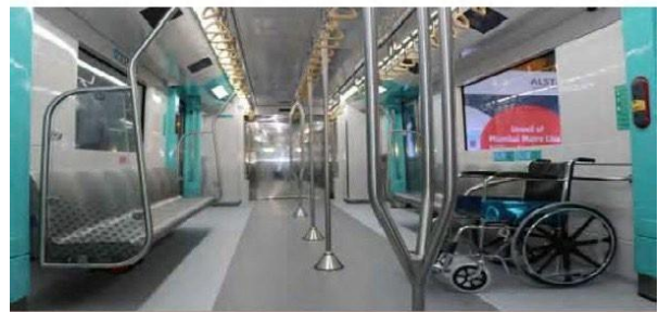
Grab poles and handrail systems
