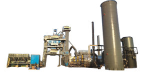
Asphalt Batch Mixing Plant
