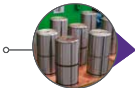
Finished products after Induction Heating and Quenching (IHQ)
