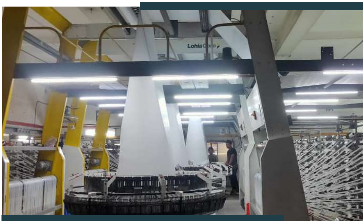
Circular weaving loom Nova 81 by LohiaCorp circular weaving machine, exemplifying our focus on precision, efficiency, and advanced manufacturing technology.
