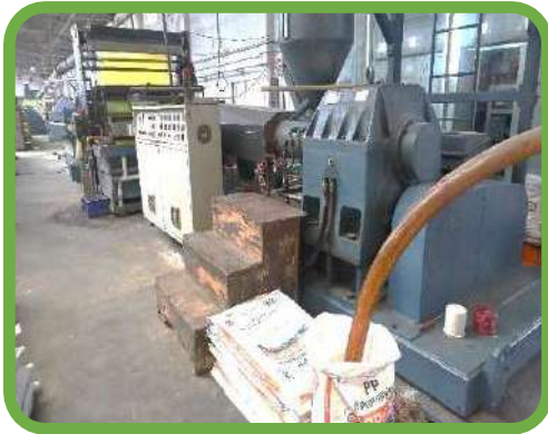
Raw materials are fed into extruder
