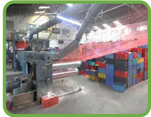
Film getting slit into strips (tapes)
