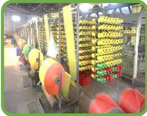
PP Strips (tapes) Bobbins are fed on the loom and Leno fabric is manufactured by weaving and then fabric is rolled in a roll
