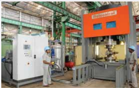
30,000 psi Hydro Test Bench for Oil Field Equipment at BHEL, Tiruchirappalli
