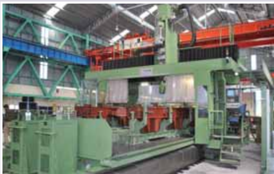
Bogie Machining Centre for AC Locomotives at BHEL, Jhansi
