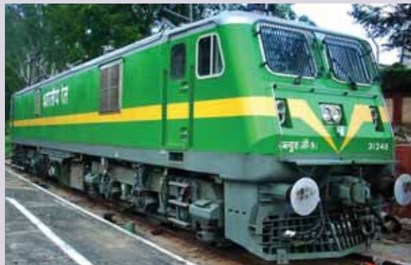
6000 hp Electric Locomotive of CLW equipped with BHEL's IGBT-based traction & auxiliary converters
