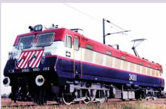
Electric Locomotive (25 kV AC, Type WAG 7)
